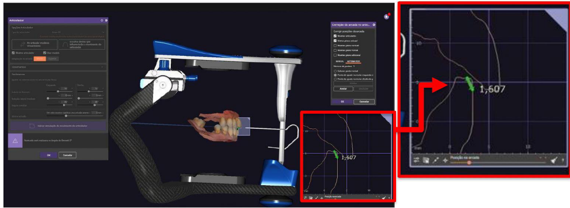
Figure. 6 – Simulation of Bennett movement and displacement tracking in exocad virtual articulator.
